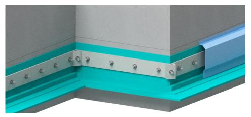
• Internal waterstops must be secured in their position before the concrete pour at an angle > 10 °.
